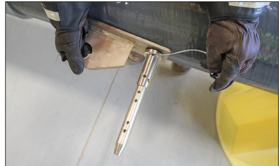
Figures 10a and 10b: Installing the Retention Collar and Determining the Correct Set of Holes for a Tight Fit
