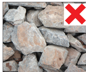
Figures 29a, 29b, and 29c: Examples of Acceptable and Unacceptable Backfill Options
