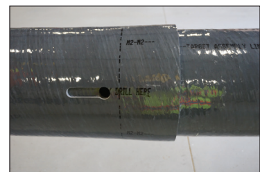
Figure 16c: Drilled Blind Nut Hole
