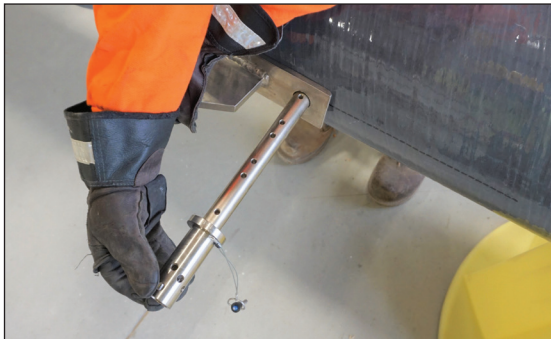
Figures 10a and 10b: Installing the Retention Collar and Determining the Correct Set of Holes for a Tight Fit
